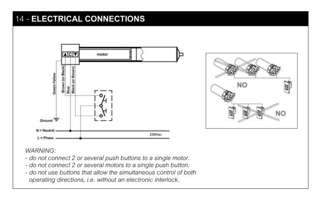
13. Disconnect mains power supply, connect motor cables to the mains power supply and to the switch, please follow carefully the instructions scheme 14. In case of using a remote control system, please follow carefully instructions contained into the radio control kit, item number no. 592 KRM00.1.
