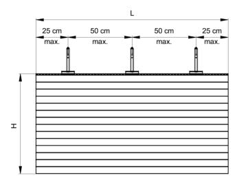
In case of wooden shutter, use the slotted clips for strap fastening (10) instead of springs (9). Check for integrity of existing strap and join it in the slotted clip holes (10) adjusting the length for obtaining the same distance from the top of the shutter for each clip.
