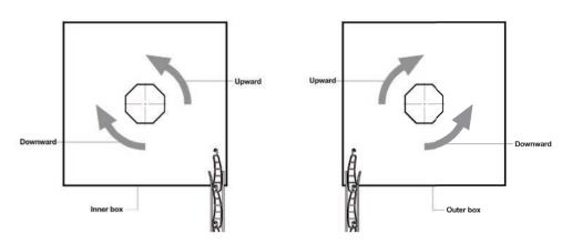
to hooking the shutter, act on the switch button for rotating the motorized tube in the sense of descent until automatic stop due to the internal limit switch, (motor will do 1 or 2 turns). In case of reverse rotation, disconnect the mains power supply and reverse brown and black cables in the switch connections.
